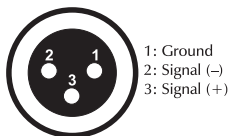
DMX-output XLR mounting-socket:
