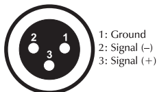
DMX-output XLR mounting-socket:
