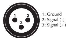
DMX-input XLR mounting-plug:
